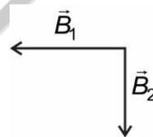
$$\text{Here, } B_{\text{net}} = \sqrt{B_1^2 + B_2^2}$$
