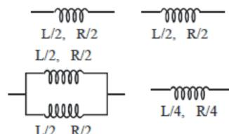
$$L_p = \frac{L_1 L_2}{L_1 + L_2} = \frac{L}{4}, \quad R_p = \frac{R_1 R_2}{R_1 + R_2} = \frac{R}{4}$$
